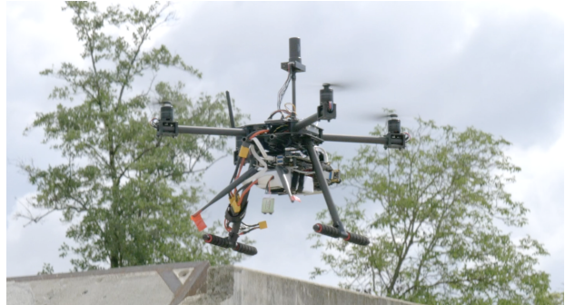
Figure 1. MAV capable of fully autonomous flight with on-board perception during a 3D reconstruction experiment.
