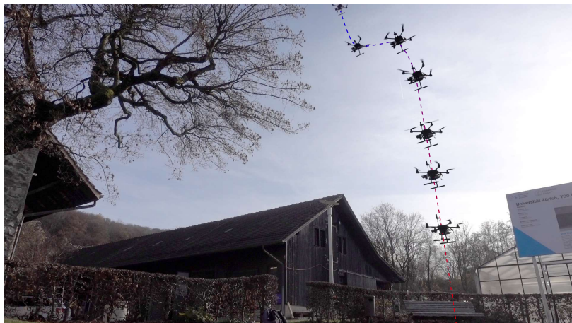
Figure 8.1: Safe emergency landing performed during a real-world experiment. Using semantic and depth information, the multi-rotor UAV finds a safe landing area and autonomously descends towards it, while avoiding collisions with the environment.
