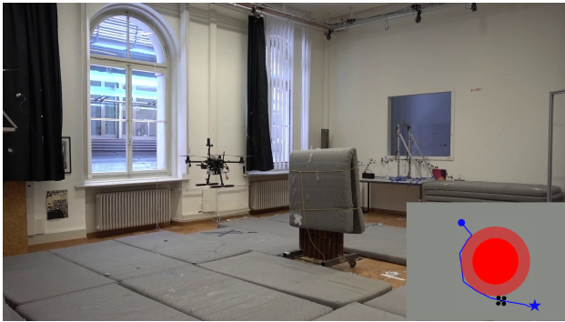
Fig. 6. Snapshot of the real-life experiment with a static obstacle, modeled as a pillar. A safety margin of 0.5m, shown as a semi-transparent rim in the inset, is added to the static obstacle. The starting position is shown as a blob, while the destination as a star.
