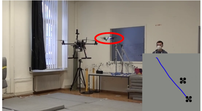
Fig. 1. Experiment with two UAVs flying in the same workspace. T-PRM successfully navigates one UAV to its destination, avoiding collision with the second, moving UAV, modeled as a spherical obstacle and highlighted with a red ellipse in the image. Our algorithm performs re-planning online, continuously adjusting the first UAV’s trajectory to the newly estimated velocity of the obstacle.
