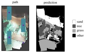
(b) As a better comparison to the IPP experiment, we start small lawnmower missions at different locations distributed over the whole map. Each mission starts at one of the blue dots and executes a rectangular pattern around this position.
