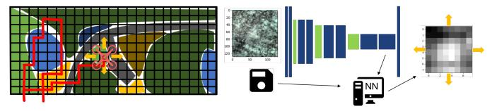
Fig. 2: Illustration of the path planning scenario. Left. The UAV is in between its mission to collect useful new training data. The path is planned as a sequence of grid cells on the map. **Right.** The current image seen from the UAV is put through the CNN to get a heatmap of patchwise novelty scores. The heatmap is then used to select the most promising next gridcell.
