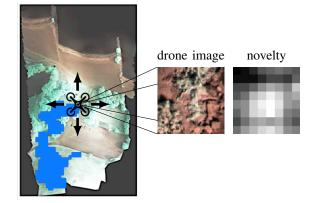
Fig. 1: To collect useful training data for a semantic segmentation network, our informative path planning algorithm finds a path for the drone that increases the novelty of the observed images. The novelty is evaluated in a patchwise manner that additionally gives directional information from the gradient over the heatmap. Brighter novelty is higher. The planned path is marked in blue.
