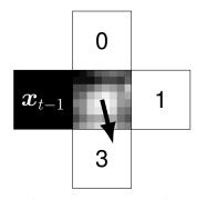
Fig. 3: Example of the gradient propagation. The UAV came from cell  $x_{t-1}$  and obtained an image in the center cell  $x_t$ , which is used to produce the shown novelty heatmap. As the novelty of the adjacent cells is still unknown, we infer information from the gradient (black arrow) of the novelty heatmap  $\nabla D(x_t)$ . A score is assigned to each of the neighboring cells and is then substracted from the potential field.
