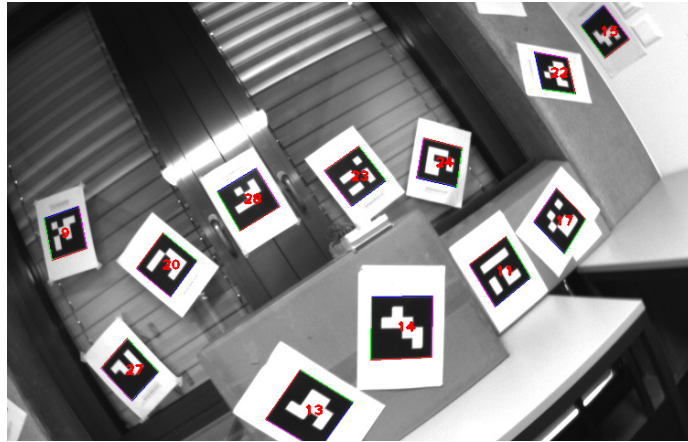
Figure 4.5: The detections of the AprilTags for one frame
