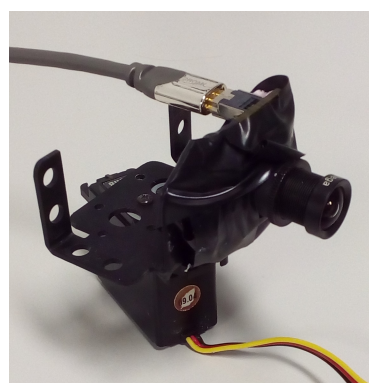
Figure 3.3: The complete system camera-servo
