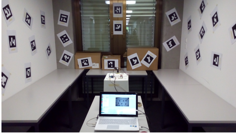
Figure 4.4: Set-up of the tags for point map creation
